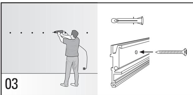
**03** Löcher bohren, Dübel einsetzen. Schiene in Dübel festschrauben. Drill holes and insert anchors. Fasten the rails to the wall using the anchors and screws.
